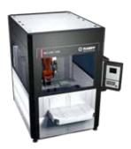
MC-CNC 1000 Robot with MS-C mixing system, double sliding table
