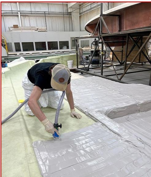
RAMPF RAKU<sup>®</sup> TOOL Close Contour Pastes are two-component epoxy systems designed for direct application to near-net-shape substrates such as EPS, wood, and the RAMPF styling board RAKU<sup>®</sup> TOOL SB-0064. This significantly reduces material consumption, production waste, and machining time for milling and finishing.
