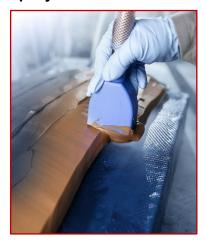
RAMPF RAKU® TOOL epoxy Close Contour Pastes are ideal for large-scale model construction, enabling cost-effective and time-saving manufacturing processes. The innovative two-component systems are applied to near-contour substructures using mixing and dispensing systems, either manually or with a CNC machine.
