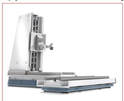
The foundation for the long-term precision of the MCµ lies in its inherent structural stability. This includes high guide bars and FEM-optimized structures cast with EPUMENT® mineral casting. The high-performance material from RAMPF Machine Systems ensures maximum stability in ultra-precise machines: Comparative measurements show that mineral casting offers up to ten times the material damping of gray cast iron and welded constructions.
