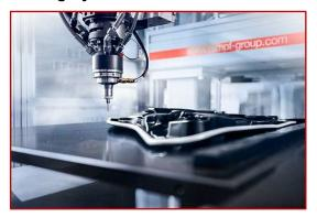
Sealing systems based on polyurethane (RAKU® PUR) and silicone (RAKU® SIL) ensure efficient and long-lasting sealing, meet the highest quality standards, and are easy to process. The fast-curing, low-emission, and heat-resistant systems protect battery covers, charging stations, and charging plugs from dust, dirt, moisture, chemical substances, and environmental influences.
