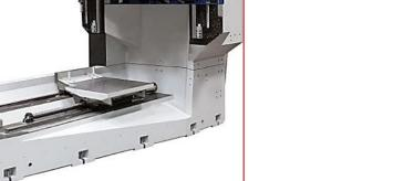
RAMPF Machine Systems supplies the machine beds for the REIDEN RX10 as a complete system. For this, the two-part machine bed is bonded using RAMPF's in-house joining and bonding technology.
