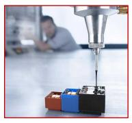
RAMPF processes reactive, thermally and electrically conductive polymers using its own premium mixing and dispensing systems, which ensure the precise and fast processing of highly filled materials. The
