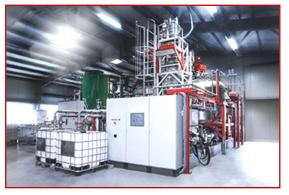
Multifunctional recycling plants designed by RAMPF Eco Solutions enable customers with high residual volumes to produce their own recycled polyols. This significantly reduces raw material, transport, and disposal costs and makes production more environmentally friendly.
