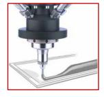
RAMPF processes multi-component reactive polyurethane and silicone foams into gaskets using multi-axis robots. After curing, a seamless gasket (formed in place foam gasket, FIPFG) is bonded to the component and provides static protection against dust and moisture. The foams can also be dispensed into a carrier mold and processed further as a custom-fit, cured gasket (molded foam).
