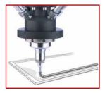
With dispensing technology and robot-assisted automation solutions, polyurethane and silicone sealing beads are applied to a wide variety of components. After curing, a non-detachable, elastic gasket (formed in place gasket, FIPG) is bonded to the component and provides static protection against dust and moisture. Flexible production systems with surface activation for improving adhesion,
