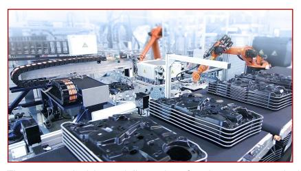
The automated mixing and dispensing of gaskets guarantees both for efficient production processes and the long-term protection of components against moisture, dust, chemicals, and various environmental influences.
