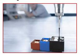
RAMPF processes reactive, thermally and electrically conductive polymers using its own premium mixing and dispensing systems, which ensure the precise and fast processing of highly filled materials. The produced parts are reliably protected from contact, moisture, and damage, guaranteeing for the lasting, high-performance functioning of electronic assemblies.
