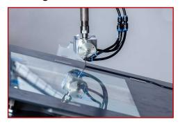
RAMPF processes multi-component adhesives into precisely reacting products for joining components. The components can be pre-treated to improve adhesion. The high-precision joining process can be carried out manually or fully automated. Integrated curing-on-demand (COD) systems accelerate the curing process. When joining components in a vacuum, products such as displays are applied without air bubbles (optical bonding).
