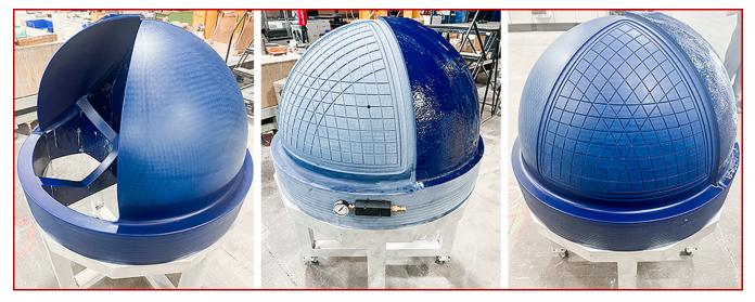
Visitors to the RAMPF booth can see for themselves the high quality which is achieved with RAMPF Close Contour Castings. Using RAKU<sup>®</sup> TOOL CC-6503, Symmetrix Composite Tooling, a full-service composite tooling manufacturer of complex and innovative designs based in Bristol, R.I., produced a lightweight sphere with first-class surfaces.
