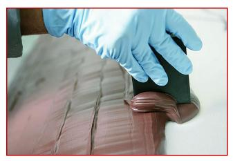
The two-component, thixotropic epoxy systems are applied to a close-contour shape supporting structure with a mixing and dispensing machine, cured, and then CNC machined according to customer CAD data; almost any kind of supporting structure can be used, including RAKU® TOOL SB-0080 styling board, EPS, and cast aluminum.
