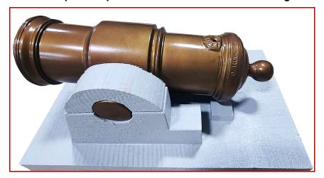
Due to the prohibitive cost of reproducing period-correct bronze cannon tubes, RRNBP reached out to RAMPF Group, Inc. to manufacture models of the canon using a silicone mold and polyurethane resin. The company based in Wixom, MI, is renowned for its tooling expertise and first-class portfolio of board and liquid materials for state-of-the art modeling. For the cannon project it had the perfect products on hand – the tin silicone RAKU TOOL® RS-9225 and the rigid polyurethane RAKU TOOL® IE-3082.
