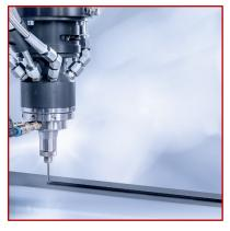
> FIPG and FIPFG foam gaskets: RAMPF manufactures custom-made formed in place gaskets (FIPG) and formed in place foam gaskets (FIPFG) made of polyurethane using speed-robotic CNC dispensing. The foam gaskets are applied directly to the component of the customer, expand in situ, and bond very quickly, reducing cycle times and ensuring efficient processing.
