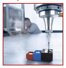
RAMPF processes reactive, thermally and electrically conductive polymers using its own cutting-edge mixing and dispensing systems. These ensure the precise and fast processing of highly filled materials. The produced parts are reliably protected from contact, moisture, and damage, guaranteeing for the lasting, high-performance functioning of electronic assemblies.
