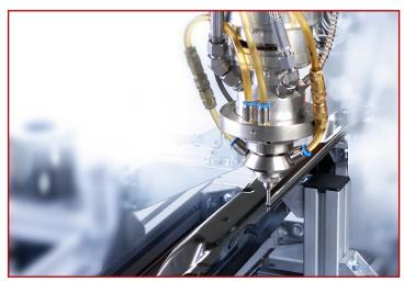
Liquid to highly thixotropic and compact gaskets based on polyurethane and silicone offer maximum and long-term protection against moisture, dust, and chemicals.
