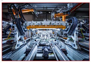
Customized, highly automated turnkey production systems with integrated dispensing technology for sealing, casting, and bonding make manufacturing battery packs an ultrafast, high-precision process.
