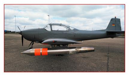
Equipped with a spraying mechanism, the Reutlingen association's cloud seeding aircraft is based at Stuttgart airport. The pilots spread a mixture of silver iodide and acetone under the clouds. Updrafts then transfer the mixture into the storm clouds. This prevents large hailstones from forming, and although more hailstones are created in total, they are much smaller, and therefore cause less damage. © Markus Duwe
