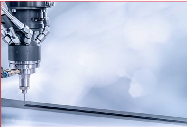
What's more, RAKU® PUR 32-3294-2 boasts an impressive economic advantage – thanks to its very low density, a minimal amount of material needs to be used. The integral RAKU® speed technology means the material is tack-free at room temperature in a very short time, so cycle and handling times are extremely fast.
