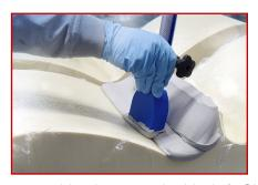
Close Contour materials include Close Contour Pastes (two-component epoxy systems which are applied to a close contour substructure by hand or CNC machine), Close Contour Castings (semi-finished polyurethane products supplied as three-dimensional castings that are already close to the final contour), and Close Contour Blocks (polyurethane or epoxy systems which are produced to customer specifications and delivered as
