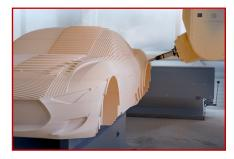
**Tooling boards** made from polyurethane and epoxy exhibit outstanding mechanical properties, finest surface structures, and good dimensional stability. The boards are easy and quick to machine and compatible with all industry-standard paints, release agents, and epoxy prepregs. RAMPF boards are used, amongst others, for the manufacture of styling, master, cubing, and presentation models, negative
