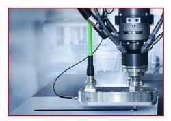
The MC dispensing machine is equipped with RAMPF's modular microwave technology RAKU® Microwave Curing. Attaching an applicator below the mixing head of the dispensing system further heats the reactive mixture via microwaves, speeding up the system and thus ensuring the casting resin cures faster. The key advantage – one- and two-component electro casting resins react up to four times faster, which means that the component can be load-
