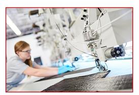
The advantages of TFP for lightweight construction using composites are striking – mass-specific stiffness and strength are maximized by selectively placing and orienting the carbon fiber and fiberglass filaments where strength or weight optimization is required. The structural performance of the composite is maximized while also providing for greatest possible weight savings, reduced carbon fiber usage, and lower cost.
