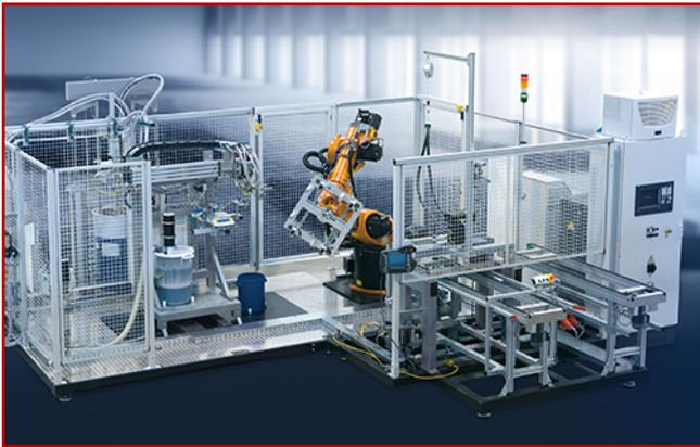
The C-DS compact dispensing system is designed for processing one- and two-component adhesives, casting, and sealing materials. The system is highly versatile and can be used in manual workstation or fully automated robot systems.
