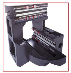
Outstanding vibration damping, high degree of functional integration, sustainable and environmentally friendly production – the machine bed of this high-speed milling machine is made from RAMPF EPUMENT® mineral casting.
