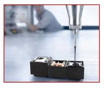
RAMPF casting systems based on polyurethane, epoxy, and silicone ensure optimum heat dissipation in batteries and power electronics, while providing long-term protection against chemical substances and environmental influences. This maximizes service life, reliability, and performance. Gap fillers and heat-conductive casting materials guarantee optimized heat management of electrical and electronic components.
