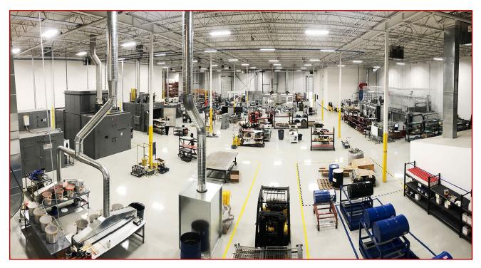
In RAMPF Composite Solutions' new facility in Burlington, Ontario, engineered solutions in advanced carbon fiber and fiberglass composites are manufactured using cutting-edge technologies. Core competencies include composite manufacturing to very tight tolerances utilizing the out-of-autoclave VARTM process, resin infusion, metal plating, and value-added assembly.
