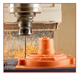
King of abrasion resistance – RAMPF Tooling Solutions' foundry board RAKU® TOOL WB-1258 produces an unrivalled high number of parts, previously only possible when using liquid systems. It is well suited to replace metal tools in foundry applications as it has a number of key advantages, including its much lower weight, excellent machinability, and the fact that changes can be made easily. Applications include pattern plates and core boxes.
