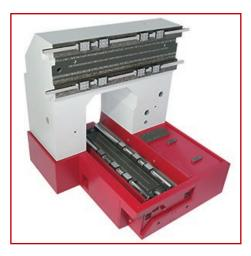
EPUMENT<sup>®</sup> mineral casting from RAMPF Machine Systems consists of selected minerals and stones and high-quality epoxy resin-based binding agents. The key advantage over gray cast iron and welded constructions is the considerably enhanced damping, which ensures the machine bed structure has greater dynamic stability in ultrafast and high-precision production machinery.
