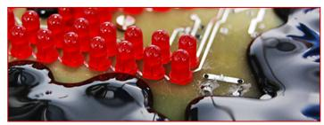
Electro casting resins from RAMPF Polymer Solutions provide sensitive electrical and electronic components with reliable and efficient protection against chemical substances and environmental influences such as heat, cold, and moisture. They therefore ensure the parts' better performance, longer service lives, and greater cost-efficiency.
