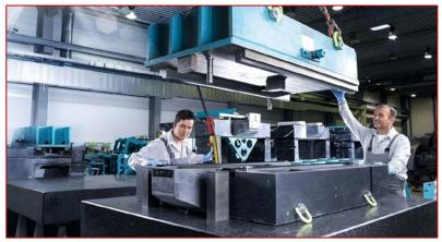
Another benefit of EPUMENT mineral casting is the high production efficiency. With RAMPF's cutting-edge molding technology, a flatness and straightness of 0.02 millimeters are achieved over a replication length of four meters. Accuracies in the hundredths of a millimeter range could previously only be reliably achieved with molding lengths up to 2.5 meters.
