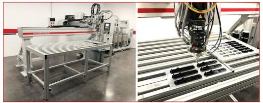
Ideal solution for complex requirements: Sellados Industriales is using the DR-CNC dispensing robot from RAMPF Production Systems.
