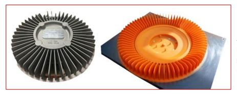
At GIFA 2019, RAMPF Tooling Solutions is showcasing a RAKU® TOOL WB-1258 pattern plate used to produce a fan housing.
