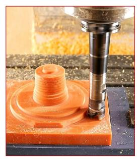
Thanks to its exceptional abrasion resistance, more than 100,000 replications can be produced with the polyurethane board RAKU® TOOL WB-1258. This was previously possible using either liquid systems with complex manufacturing processes with higher costs or high-priced metals like aluminum.
