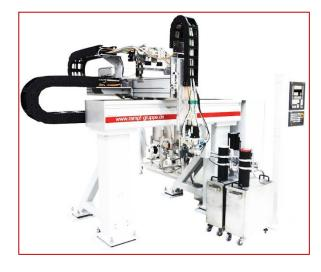
The dispensing robot DR-CNCe was specially developed for the markets in Asia and the Middle East. With its variable X-Y-Z strokes, the DR-CNCe offers highest flexibility for the three-dimensional dispensing of sealants, adhesives, and casting systems. The mixing and dispensing technology forms the basis for highly automated production systems for individual customer projects.
