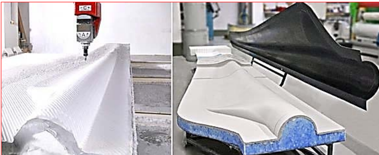
This mold for producing wind turbine blades using the composite construction method was manufactured using Close Contour Paste RAKU ® TOOL CP-6060.
