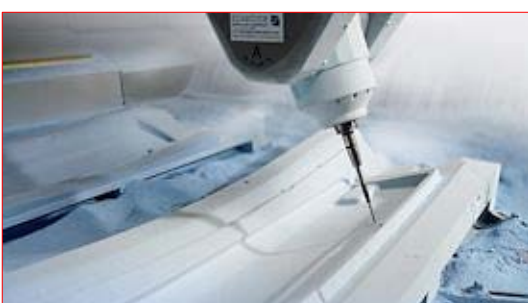
Milling of a prepreg lay-up tool from RAKU ® TOOL WB-0691 for composite part production.
