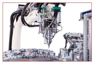
The fully automated cell for PU bonding exterior car parts developed by RAMPF Production Systems maximizes the speed, precision, and flexibility of production processes.
