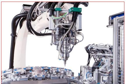
The fully automated cell for bonding exterior car parts developed by RAMPF Production Systems maximizes the speed, precision, and flexibility of production processes.
