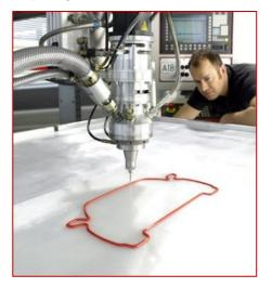
RAMPF manufactures custom-made FIPG (formed in place gaskets) and FIPFG (formed in place foam gaskets) made of polyurethane using speed-robotic CNC dispensing. The foam gaskets are applied di-
