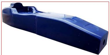
For this monocoque body of a racing car RAKU<sup>®</sup> TOOL Close Contour Casting CC/CB-6503 was used for the production of master models for prepring lay-up tools. Close Contour Castings are delivered to the customer as a three-dimensional shape that is already a close contour of the final shape.
