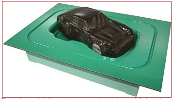
This carbon model of a sports car was produced via resin infusion using a shell lay-up tool. The surface was manufactured using RAKU® TOOL gelcoat EG-2105 / EH-2950. The backing was manufactured using RAKU® TOOL resin infusion El-2500 / EH-2970-1 / carbon fibers. The final part is made of carbon fiber with RAKU® TOOL El-2500 / EH-2970-1.
