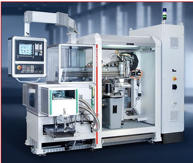
Developed for vacuum casting demanding materials – RAMPF DC-VAC Vacuum Dispensing System.
