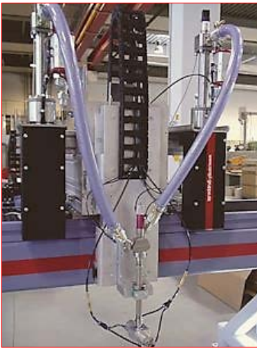
E-KDP 250 piston dispensing pump with static mixer, developed and produced by RAMPF Production Systems.
