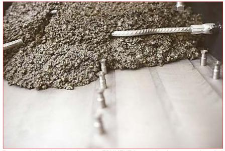
Epoxy resin-bonded mineral casting EPUMENT is used for the construction of vibration-damping machine beds and machine bed components in highly dynamic mechanical engineering applications.
