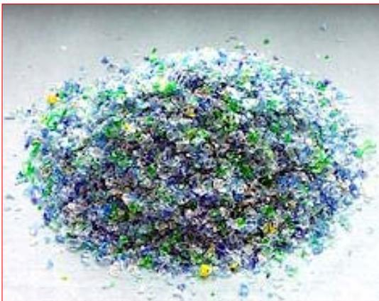
RAMPF Eco Solutions views production residues and post-consumer PET from packaging not as waste but as valuable sources of raw materials. A special chemical method is used to process these materials into polyol, which is then recycled in polyurethane.
