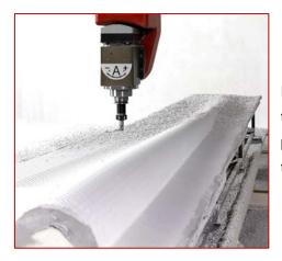
RAKU® TOOL CP-6060 Close Contour Paste was developed specially for the production of large models and molds. The paste was used for the production of this wind turbine blade model to manufacture blades using the composite construction method.
