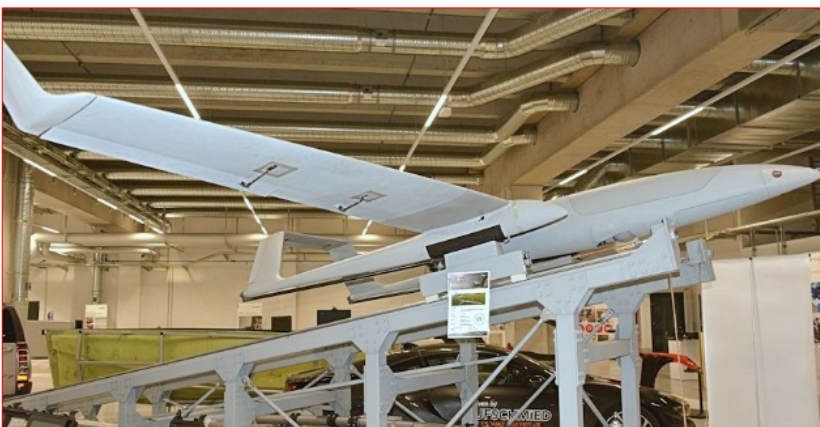
For the production of this drone, the modeling board RAKU ® TOOL MB-0600 was used for the manufacture of master models. For some of the other parts of the drone, the epoxy infusion resin system RAKU ® TOOL EI-2500 was used.
