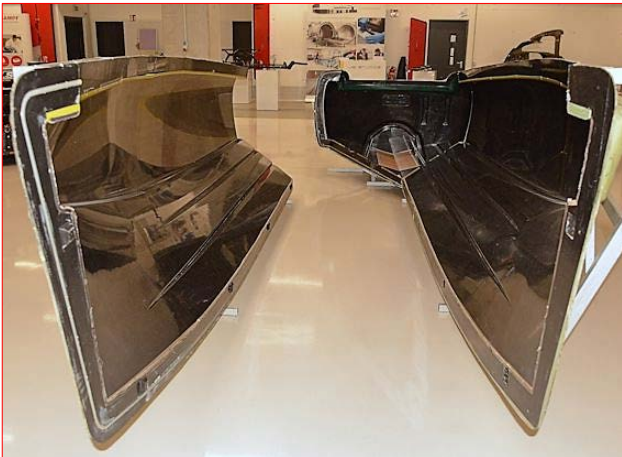
The biggest exhibit on show: This production mold for a boat hull was manufactured using resin infusion with RAKU ® TOOL EG-2104 / EH-2950-1 gelcoat resin and the RAKU ® TOOL EI-2500 / EH-2973 resin infusion system.
