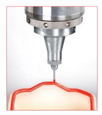
All standard polyurethane and silicone foams can be processed into gaskets using mixing and dispensing technology from RAMPF Production Systems.
