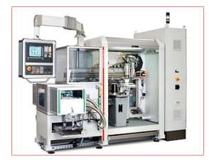
The application of the bonding material is carried out by the RAMPF DC-VAC Vacuum Dispensing System. Designed for processing one- and two-component casting materials, it is fitted with vacuum material conditioning as standard and equipped with a dynamic mixing system. The encapsulating process can be easily adjusted and monitored thanks to the large viewing window.
