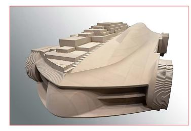
This 1:1 model of a sports car prototype was made from RAKU-TOOL<sup>®</sup> MB-0600. The polyurethane board material, which is easy to mill and process, has a very good surface structure and dimensional stability. The adhesive used is perfectly matched to the board material in density and color.
