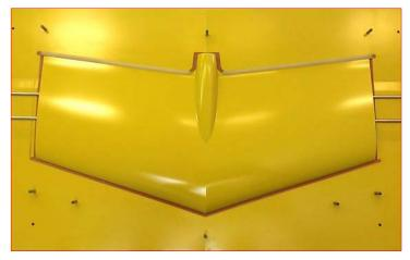
RAKU-TOOL<sup>®</sup> WB-1404 board material, RAKU-TOOL<sup>®</sup> EG-2102 / EH-2950-1 gelcoat, and RAKU-TOOL<sup>®</sup> EI-2500 / EH-2973 resin infusion system were used to produce a center wing for a model airplane.
