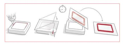
> RAKU-PUR® Perfect Fit molded sealing foam – the new and fully automated processing solution is the unbeatable alternative to cut foams. The FIPFG systems guarantee for the reliable and long-lasting sealing of parts and components in the automotive and filter industries. The shape of the gasket is based on the form and thereby free in design.
