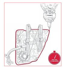
For a number of industrial applications requiring complex production lines, e.g. in the automotive industry, the component must be handled immediately after the gasket has been applied. Here, RAKU-PUR Speed technology provides an unbeatable advantage: a small curing queue and one operator are sufficient to apply the polyurethane foam gasket and ensure the components are ready for use. Multiple operators, cost-intensive curing ovens and storage systems are things of the past.
