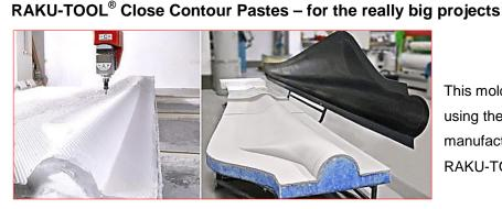
This mold for producing wind turbine blades using the composite construction method was manufactured using Close Contour Paste RAKU-TOOL<sup>®</sup> CP-6060.
