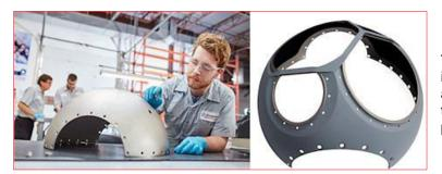
This camera gimbal is mainly employed for monitoring systems and often fitted to helicopters. All aspects of design, engineering, and manufacture are carried out in-house by RAMPF Composite Solutions.
