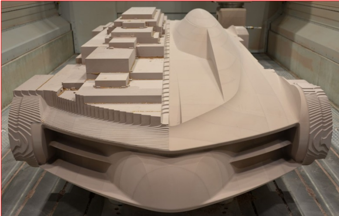
1:1 model of a sports car being milled out of RAKU-TOOL ® MB-0600 boards.
